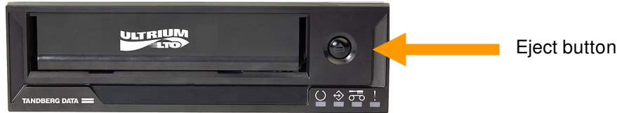
Figure 4.4 Location of the eject button
